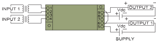
CR4640 Two Element with External Voltage Transformers * *
